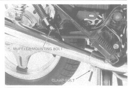
Remove the exhaust pipe clamp nuts.
